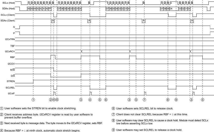
Client clears SCLREL bit. Client pulls SCLx line low to stretch clock. (5) User software reads I2CxRCV register. RBF bit clears.
