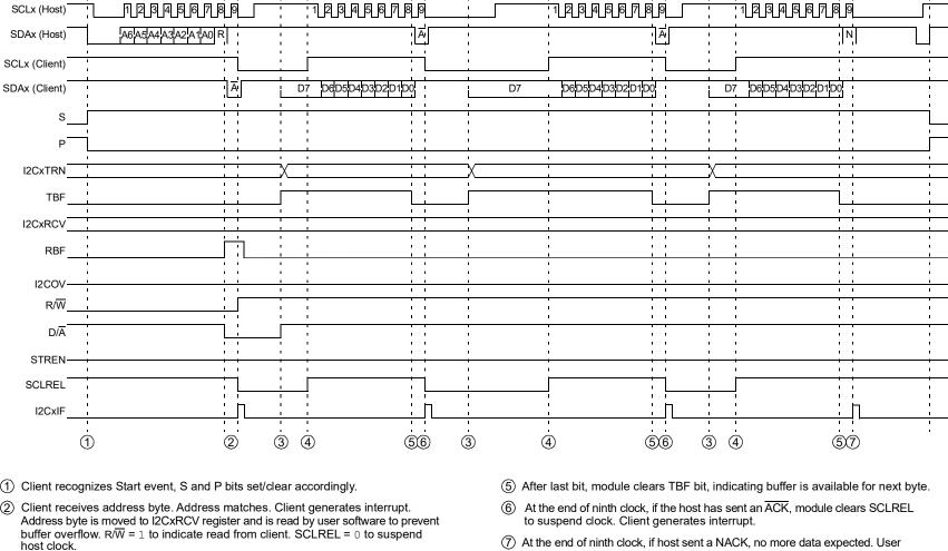
User software sets SCLREL to release clock hold. Host resumes clocking and client transmits data byte.
