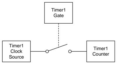
Timer1 Gate connects the clock source to the timer which will subsequently start counting. This method only concerns itself with closing and opening the gate.
