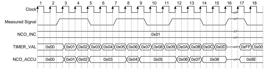
When the signal is high and on the clock's rising edge, the NCO increments its accumulator value by 1. The timer is continuosly incrementing until it is disabled (not shown). The 'Measured Signal' waveform has an approximate duty cycle of 60% (3 high counts / 5 total counts). A more realistic waveform may have its period many times greater than these 5 clock counts.
