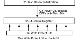
The write protect bit keeps bus masters from changing the contents of the Control register.
