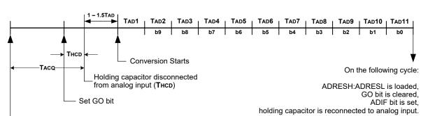
Enable ADC (ON bit)
