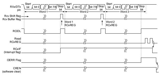
Note: This timing diagram shows three bytes appearing on the RXx input. The OERR flag is set because the RCxREG register is not read before the third word is received.
