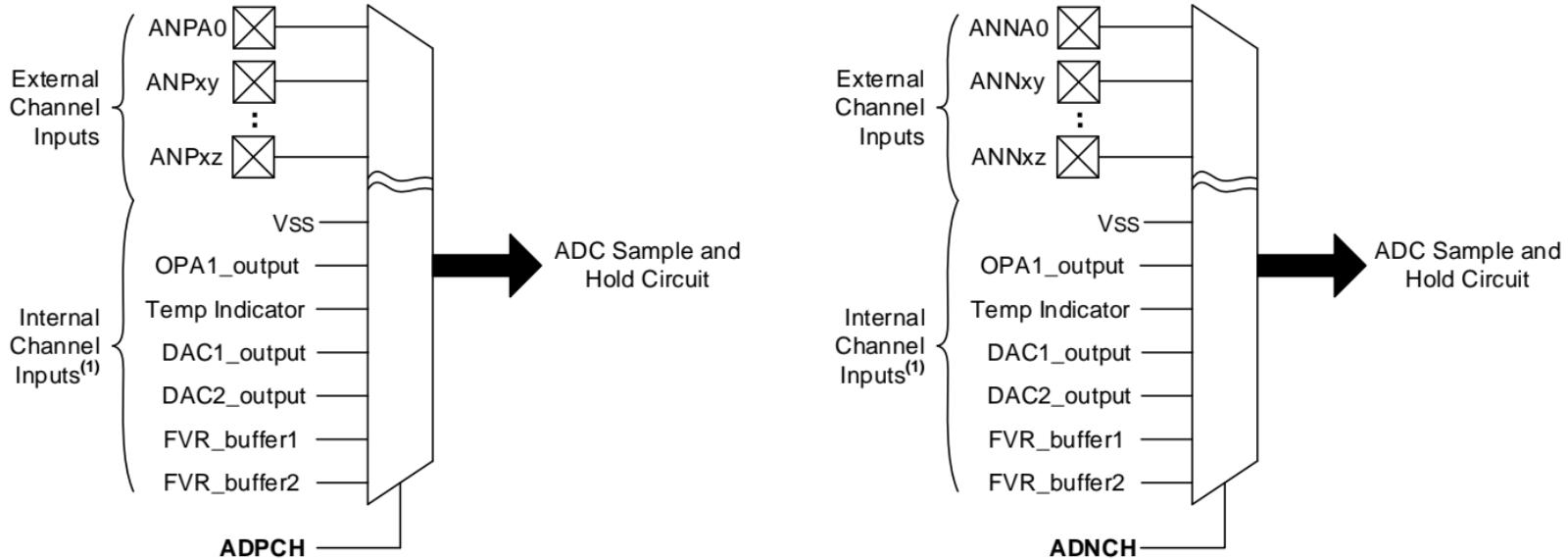
**Note 1:** The internal input channel selections vary. The inputs shown are all possible input selections. Please refer to the “**ADC Positive Input Channel Selection**” and “**ADC Negative Input Channel Selection**” tables for device-specific selection options.
