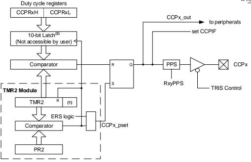
Notes: 1. 8-bit timer is concatenated with two bits generated by Fosc or two bits of the internal prescaler to create 10-bit time base.
