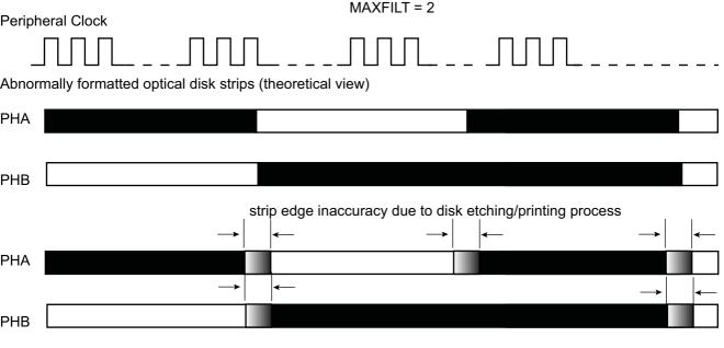
resulting PHA, PHB electrical waveforms
