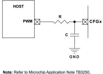
"Using PWM to Generate Analog Output" (DS90003250), for details on choosing the appropriate values of R and C.
