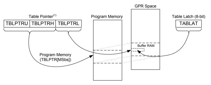
**Note 1:** During table writes the Table Pointer does not point directly to program memory. TBLPTRL actually points to an address within the buffer registers. TBLPTRU:TBLPTRH points to program memory where the entire buffer space will eventually be written with the NVM commands.
