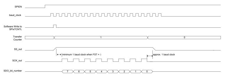
Notes: 1. SDO bit number illustrates the transmitted bit number and is not intended to imply SDO\_out tristate operation.
