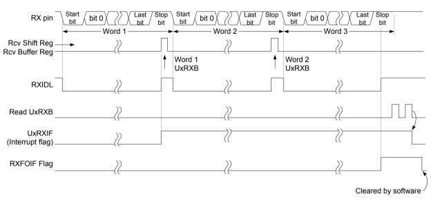
Note: This timing diagram shows three bytes appearing on the RX input. The UxRXB is not read before the third word is received, causing the RXFOIF (FIFO overrun) bit to be set. STPMD = 0, STP = 00.
