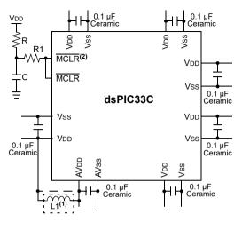
AVDD to improve ADC noise rejection. The inductor impedance should be less than  $1\Omega$  and the inductor capacity greater than 10 mA.
