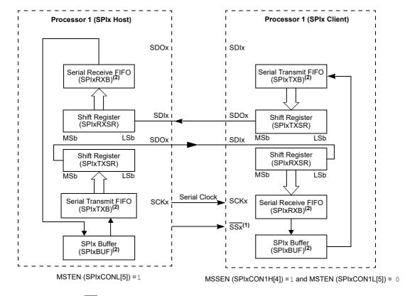
Note 1: Using the SSx pin in Client mode is optional.
