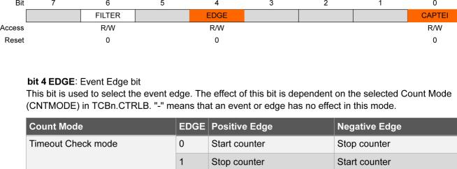
bit 0 CAPTEI: Capture Event Input Enable bits Writing this bit to '1' enables the input capture event.
