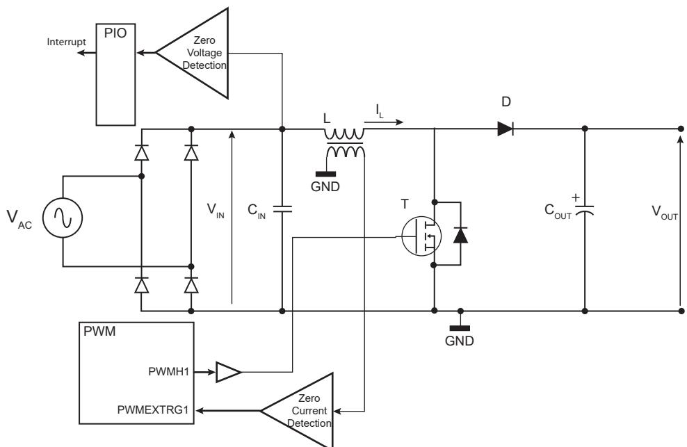
$$V_{OUT} (\text{average}) \approx \{ V_{IN\_max} * (1 + [Ton / Toff\_max]) \} - (2 \times V_{diode})$$
