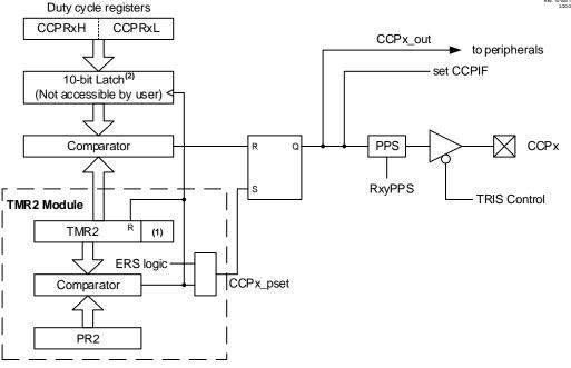
Notes: 1. An 8-bit timer is concatenated with two bits generated by Fosc or two bits of the internal prescaler to create 10-bit time base.
