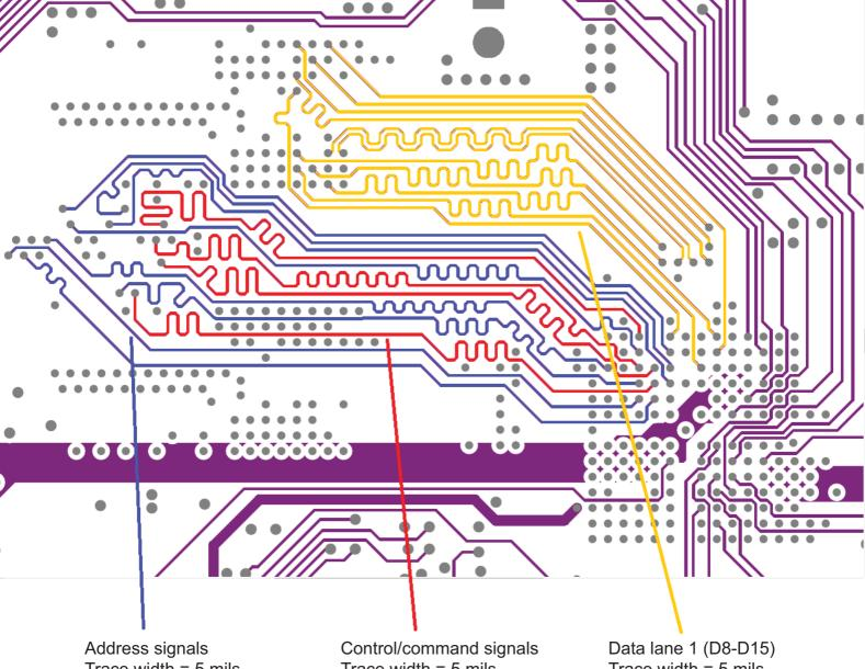
Trace width = 5 mils Trace clearance = 8 mils Control/command signals Trace width = 5 mils Trace clearance = 9 mils Data lane 1 (D8-D15) Trace width = 5 mils Trace clearance = 8 mils
