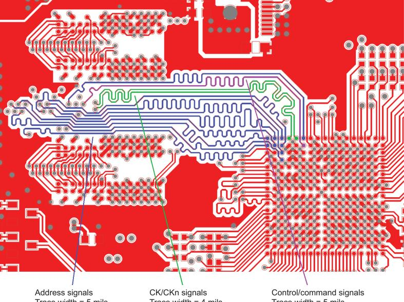
Trace width = 5 mils Trace clearance = 6 mils Trace width = 4 mils Trace clearance = 8 mils Trace width = 5 mils Trace clearance = 10 mils
