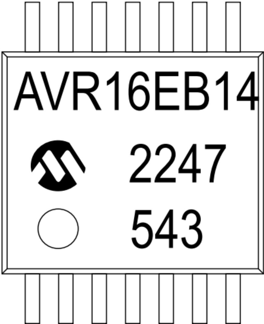
A schematic diagram of an AVR16EB14 microcontroller chip. The chip is rectangular with a double-line border. It has seven pins on the top edge and seven pins on the bottom edge. The text "AVR16EB14" is printed in a large, bold, sans-serif font across the top half of the chip. Below this, on the left side, is a circular logo containing a stylized 'A' shape. To the right of the logo is the number "2247". Below the logo is a small circle, and to its right is the number "543".
