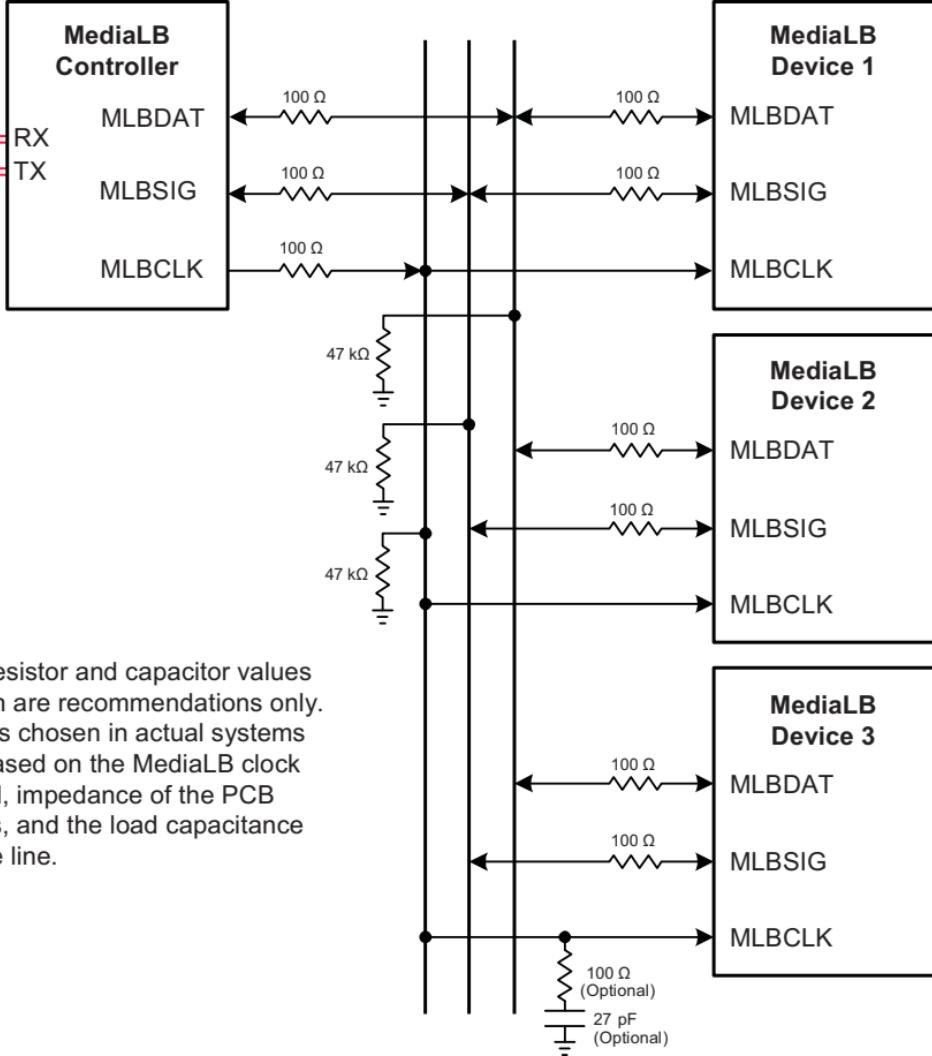
The resistor and capacitor values shown are recommendations only. Values chosen in actual systems are based on the MediaLB clock speed, impedance of the PCB traces, and the load capacitance on the line.
