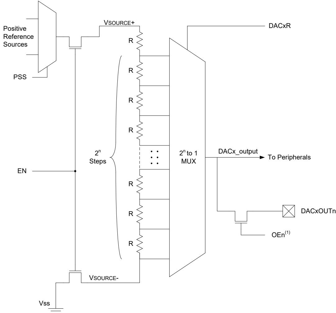
**Note 1:** The output enable bits are configured so that they act as a “one-hot” system, meaning only one DAC output can be enabled at a time.
