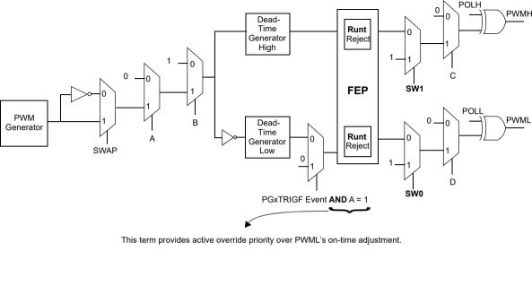
SW0 switches to tie-high when PGXIOCON1[FORCEON] = 1 AND OVRENL = 1 AND OVRDAT[i] = 1
