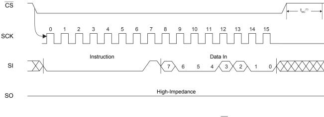
**Note:** This instruction initiates a self-timed internal write cycle  $(t_{wc})$  on the rising edge of  $\overline{CS}$  after a valid sequence.
